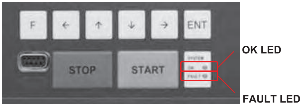
Fig. 11: Charger status LEDs
