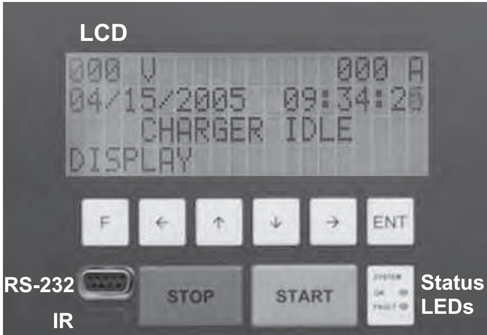
Fig. 10: LCD/Keypad and User Interfaces
